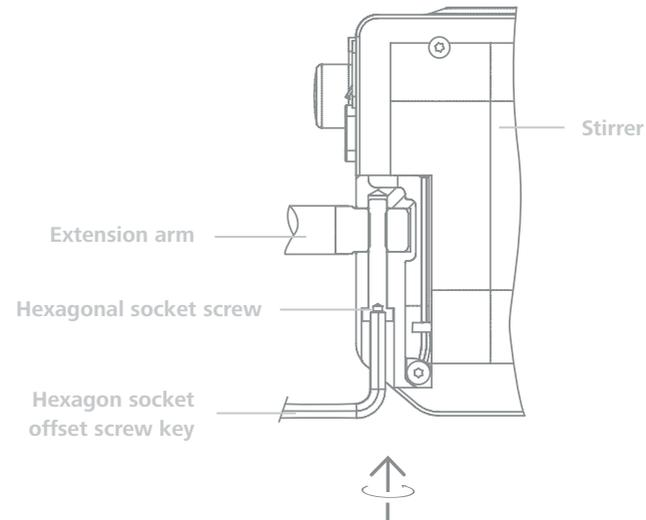
Ensure that the extension arm is fitted securely. Vibration may cause the screw to become loose. It is therefore necessary for safe use to regularly check that the extension arm is attached securely. Tighten the hexagonal bolt as required.
