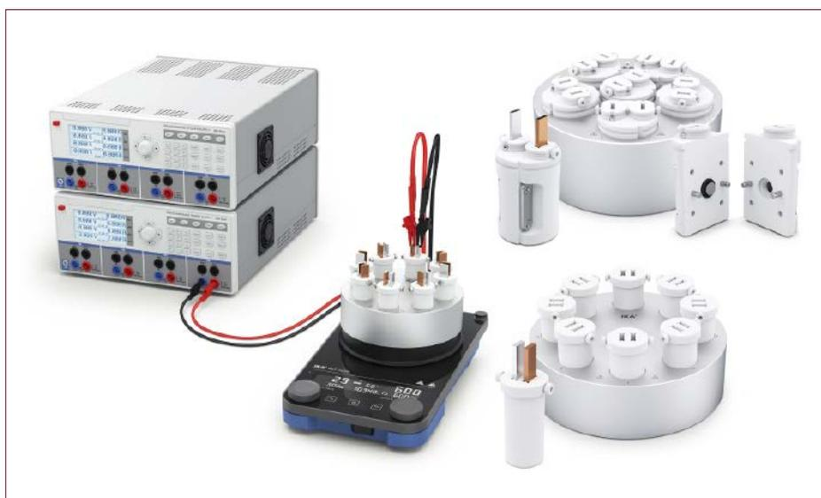
Fig. 2: IKA's commercial screening system. Left: Setup consisting of two multi-channel DC power sources, a hot plate and the reaction block including 8 undivided cells. Top right: Reaction block and single divided electrolytic cell plus two half cells. Bottom right: Reaction block and single undivided electrolytic cell.
